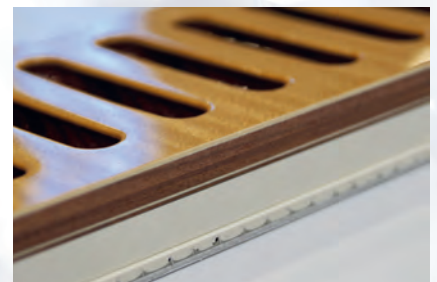
Various types of wood and veneer combined with non-wood material and milled with decorative ventilation slots before any lacquer or paint is applied, then cut to shape after surface coating on the table saw. F/LIST uses LEUCO tools.
