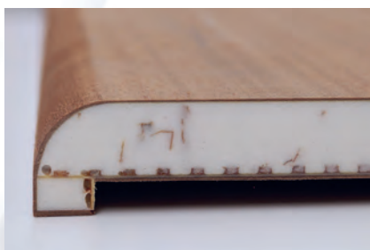
Veneered top layer and 2C edge filling, milled cleanly and without tears with the LEUCO p-System in a TRIBOS clamping fixture.
