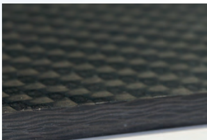
Carbon fiber materials have been in use at F/LIST for many years. F/LIST achieves smooth edges with the LEUCO p-System with a 70° shear angle.
