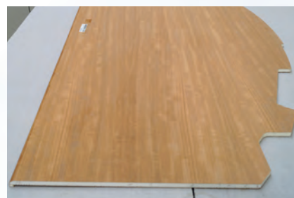
Clean edges without tears in the veneer across and along the grain, milled using LEUCO tools in a nesting process.
