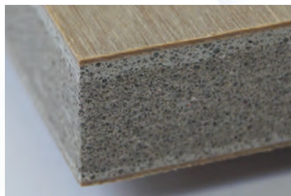
This mix of fire-retardant center layer with a high-quality top layer is almost a day-to-day routine item in the portfolio at F/LIST: In this case, abrasive blown glass was combined with a brittle veneer. The LEUCO DIAREX sizing saw blade cuts the center layer.
