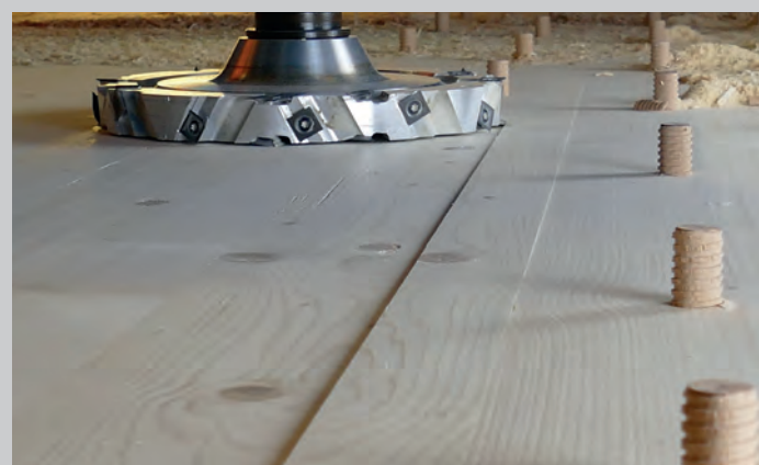
Application example for the LEUCO surfCut – plain milling of threaded connections
