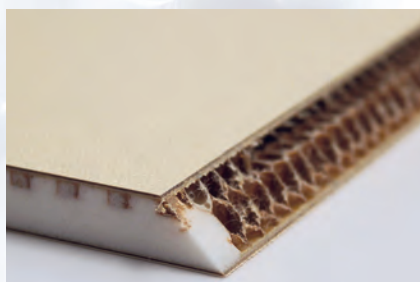
Miter cut of HPL top layers, center layer with honeycomb, two-component edge filling after the curing process: F/LIST also uses the LEUCO DIAREX saw blade for this.
