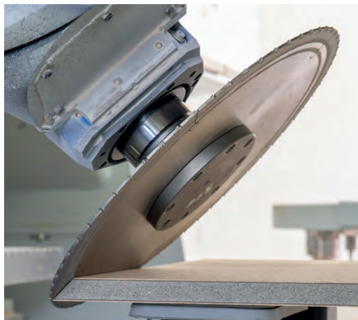
LEUCO nn-System on a CNC machine: Clean miter cut on blown glass with veneer on both sides
